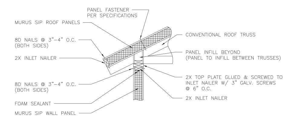
16 ROOF PANELS ON TRUSSES
